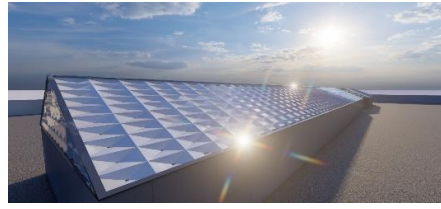
Figure 4: Dynamic louvers prevents beam sunlight (glare).
